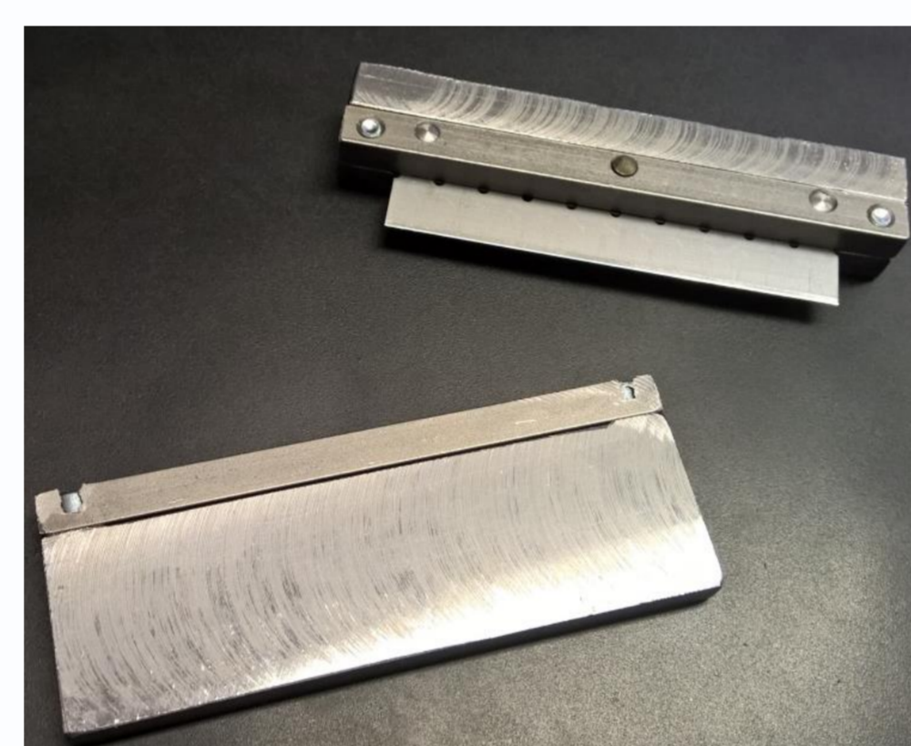
Figure 3: Microtome blade for hammer method.
